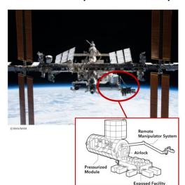
The IVA-replaceable Small Exposed Experiment Platform (i-SEEP) is JAXA's Exposed Facility for Kibo. i-SEEP can provide power and communications directly from the ISS to the payloads.
